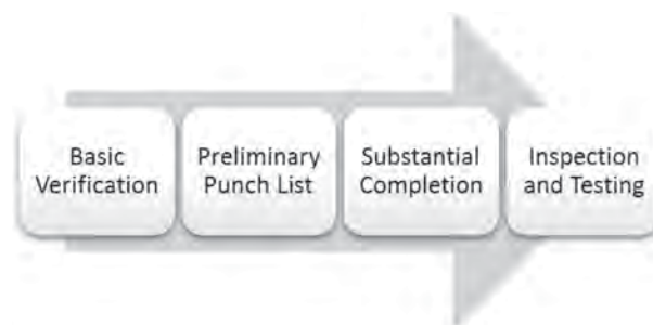
Figure 9-1. Steps in commissioning a PA system.
